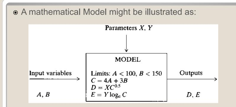
The model consists of two rules imposing limits on variables A and B, and three equations. There are two kinds of inputs: A and B are external inputs to a system, while X and Y are parameters, which are actually internal to the system, but which can be changed to calibrate the model to fit observed data
